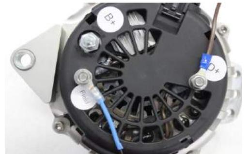
4. Ignition (White) – Connects to the ON side of the engine ignition switch which is only active when the switch in the ON position. This wire can also be connected to a switch that’s activated by engine oil pressure. This circuit must see zero volts when the engine is shut down, and battery voltage when the ignition is on and the engine is running.
