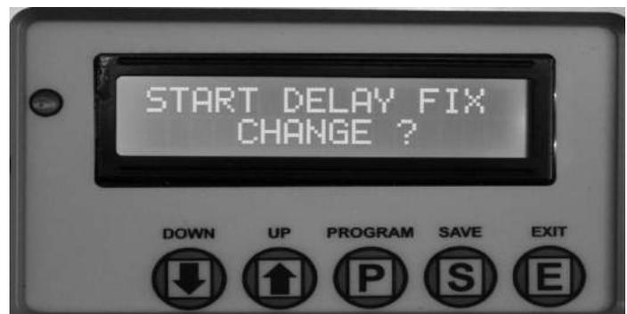
2. To change the time, press the UP button. Changes are in one minute increments. To turn off the start delay, press the DOWN button until the display reads O F F .
