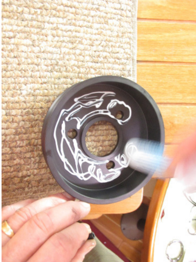
Apply Tef-Gel supplied in kit to crank pulley shive
