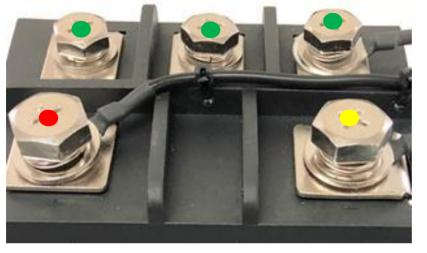
The AC connections are shown as 🔵 and the DC as (positive) 🛑 and (negative) 🥚
